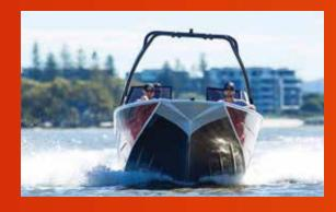
The new RSD (Raised Side Decks) featured on selected Apex models is fully-welded and increases the overall internal volume of the boat by 20%. The new RSD also increases freeboard by 80mm, offering extra comfort, safety and fishability. Combine this with a compact side deck design which maximises internal width in the Apex Hull.
